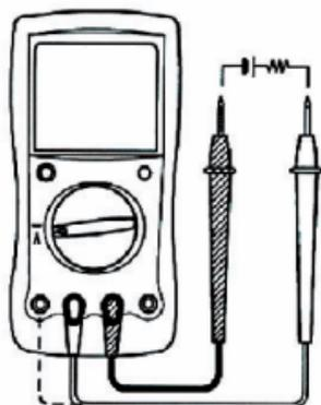
**Fig 3. Resistance measurement
