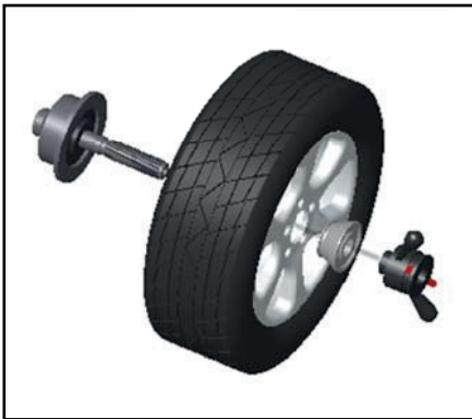
Main shaft - wheel (Installing face of rim forward inside) Cone (tip pointing to inside)-fast clamp
