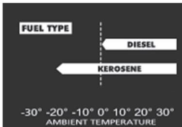
Although our heaters operate with diesel fuel, when the temperatures are below 0 °C, diesel additives are required to maintain the diesel's viscosity.
